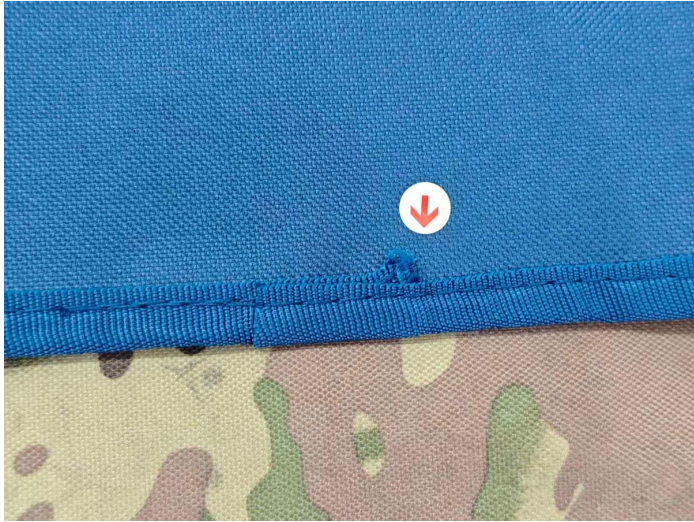
Travel Bag- Poor edge finishing-minor
