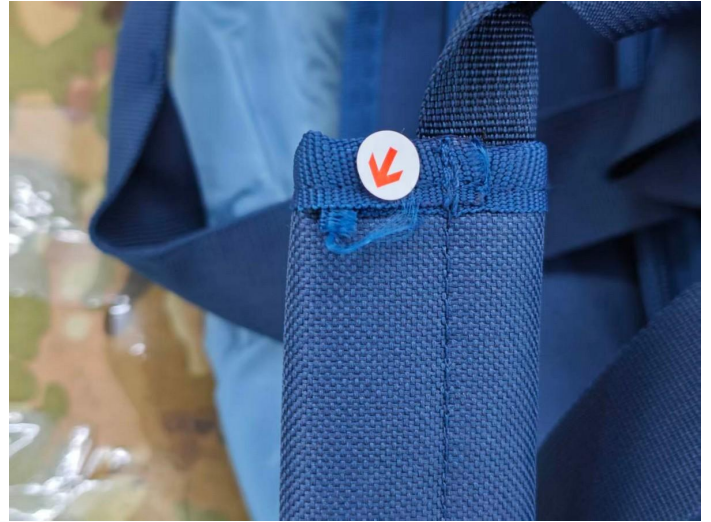
Travel Bag- Poor edge finishing-minor
